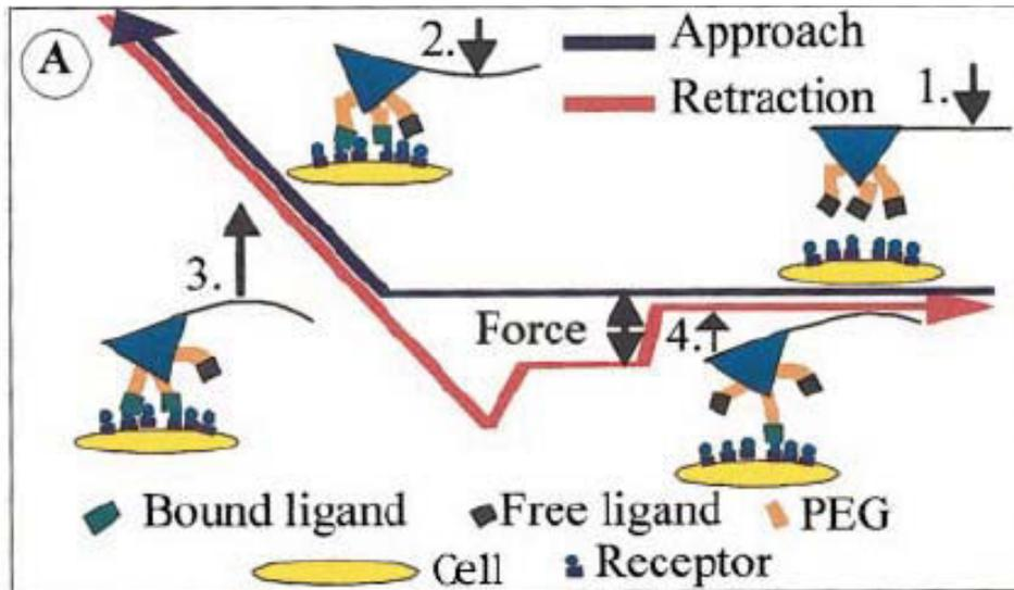
AFM used to measure the strength of integrin bonds to various RGD ligands.
