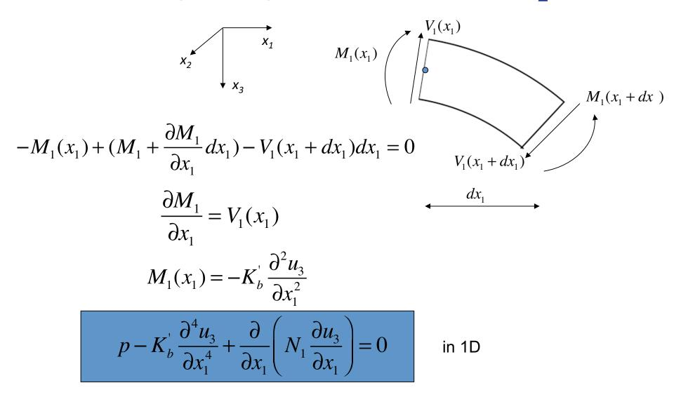
Full governing equations for linear deformations, and the reduced forms for bending or tension dominance
