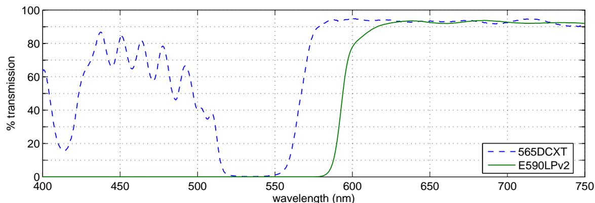
Figure 3: The transmission spectra for the 565DCXT dichroic and the E590LPv2 barrier filter.
