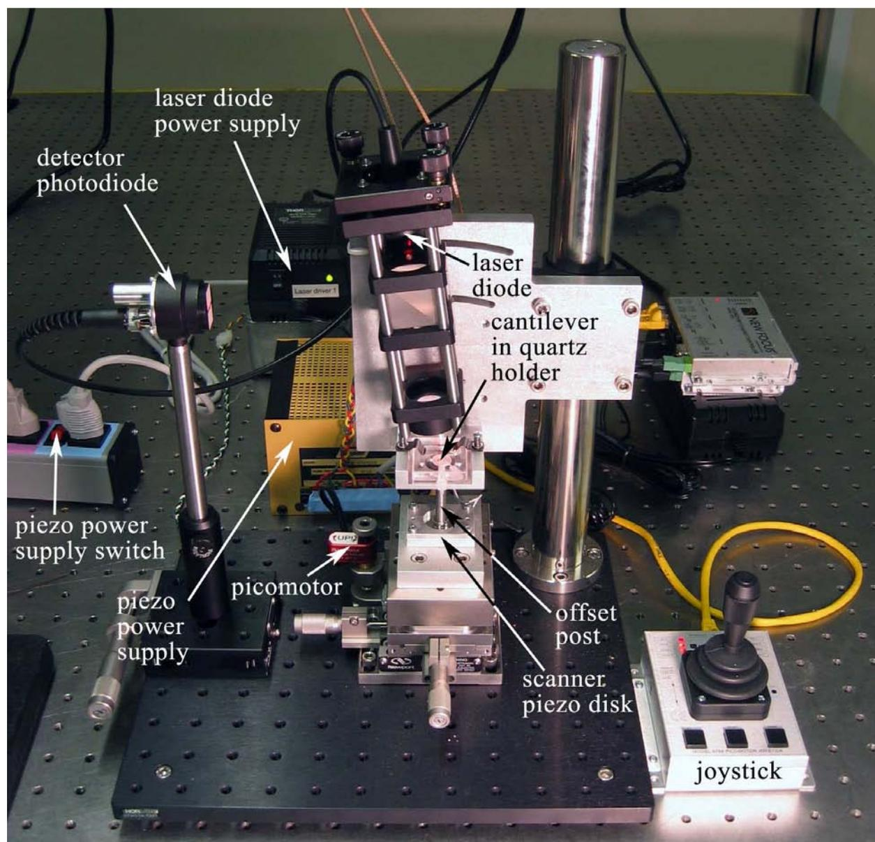
Figure 1: The AFM setup, with major components indicated.
