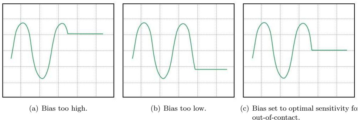
Figure 9: Proper setting of the bias point.
