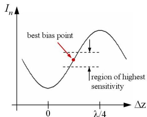
(b) The desired operating point for maximum deflection sensitivity is sketched here on the  $\sin^2$  output characteristic of the ID fingers.
