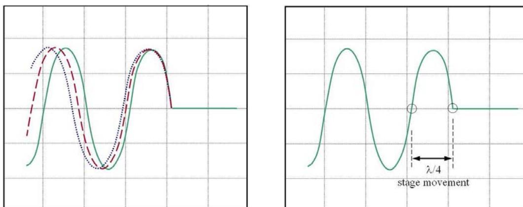
(a) Force curves for samples of varying hardness. The green (solid) curve is for a hard sample, the red (dashes) curve is softer, and blue (dots) curve is softest.
