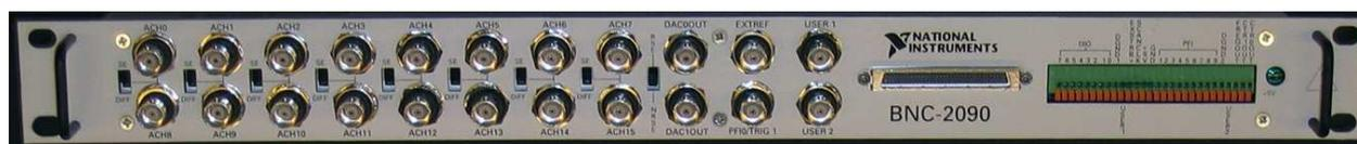
Figure 16: The data acquisition (DAQ) connection board, used for signal input and output with LabVIEW. The analog input channels are in two rows, labeled ACH0 through ACH7, and ACH8 through ACH15. The two output channels are to their right, labeled DAC0OUT and DAC1OUT, one above the other.
