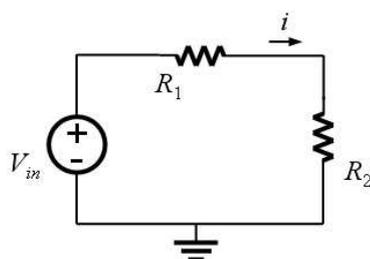
Figure 1: Resistive voltage divider circuit.
