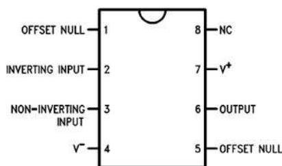
Figure 11: The pin assignments of the LM741 in a DIP-8 package.
