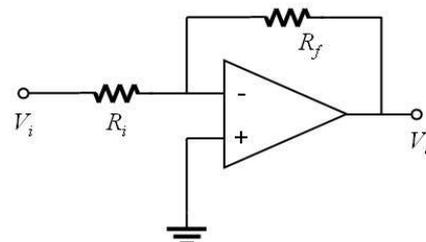
Figure 10: A basic inverting op-amp circuit.
