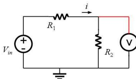
Figure 2: Measuring voltage across  $R_2$ .
