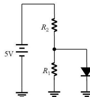
Figure 4: A voltage divider driving an LED.
