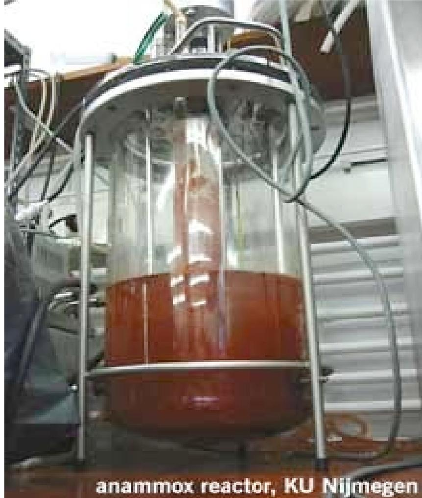
Anammox means "anaerobic ammonium oxidation". Anammox is both a new low-cost method of N-removal in wastewater treatment, and a spectacular microbial way of life - **woo - woo !**
