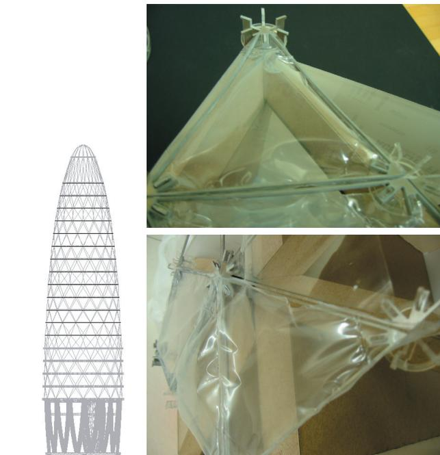
Figure 2. ETFE cushions attached to the large scale mock-up system with connection part.
