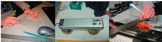
Figure 1. ETFE cushion fabrication process. After drawing specific patterns on the layer (a), Hot plate (b) was used to bond two polymer layers (c).
