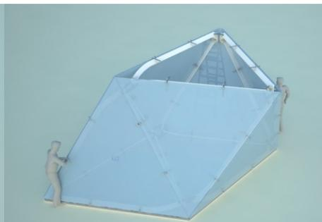
**5.** Panels are attached using spring joint system
