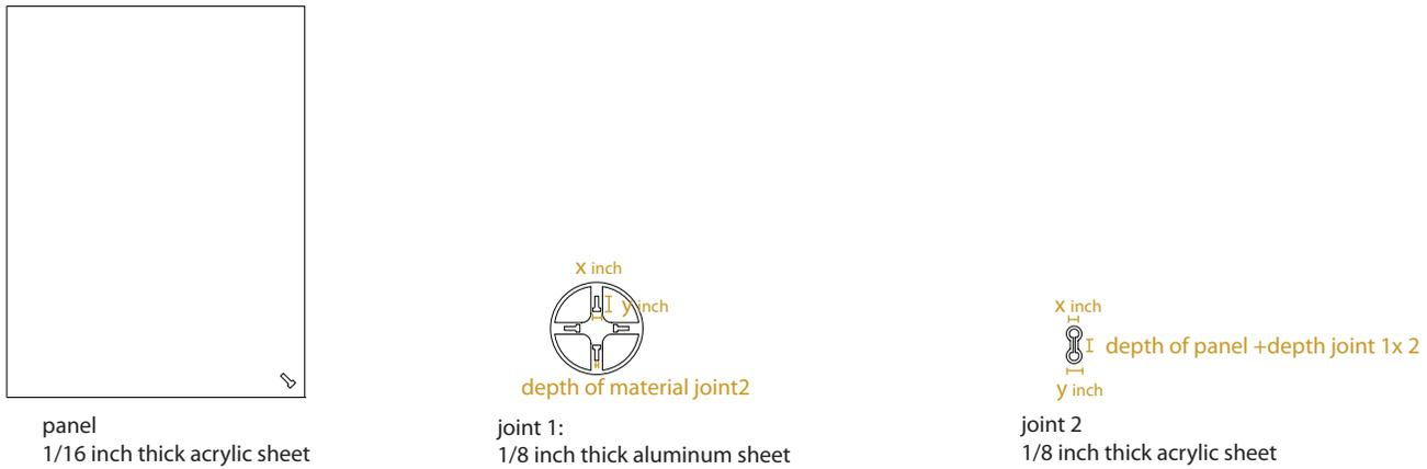
figure 1 three types of components
