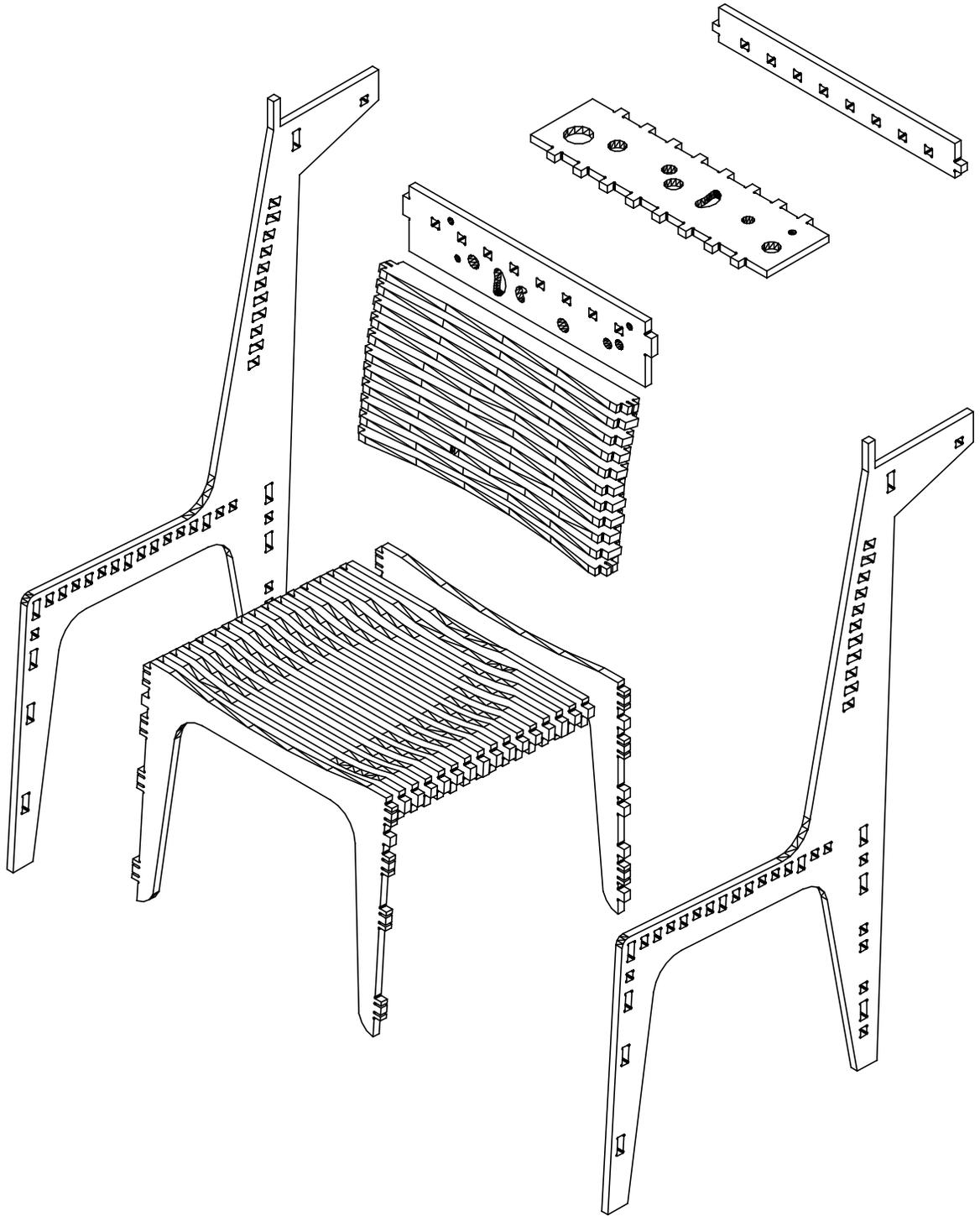
Construction model (axonometric view)
