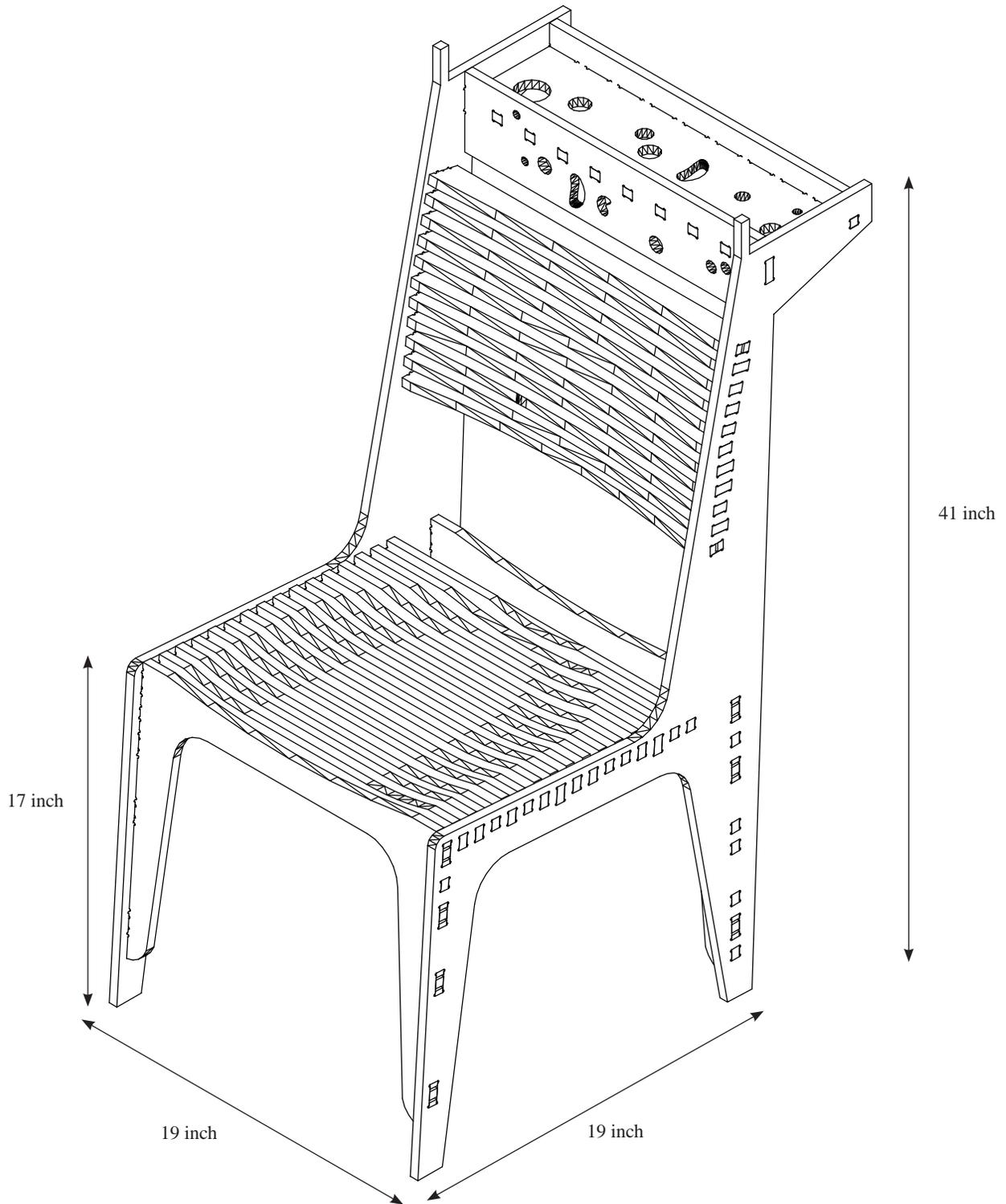
Design Model (Axonometric View)
