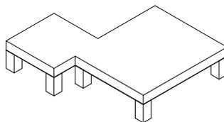
Fig. 2. 12" Floor deck over 12" square piles
