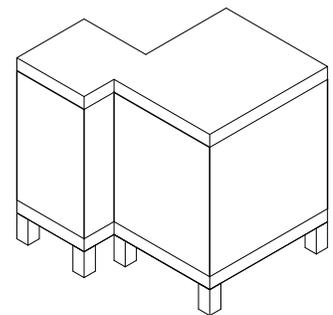
Fig. 3. Walls with a 12" thick roof deck.
