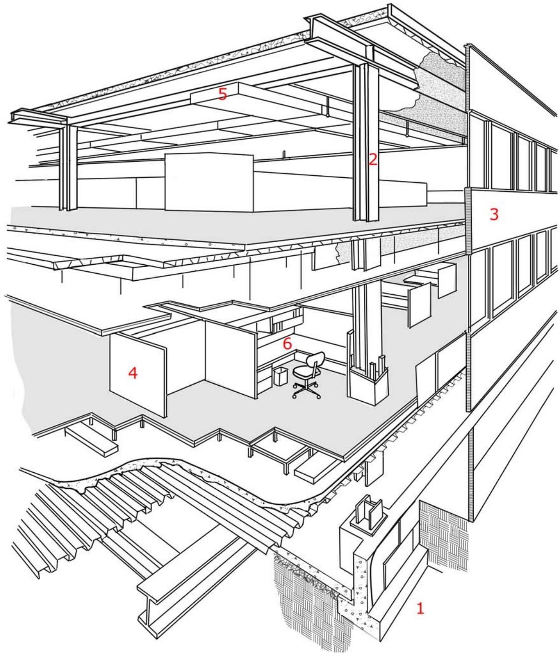
Curtainwall and raised floor construction.
