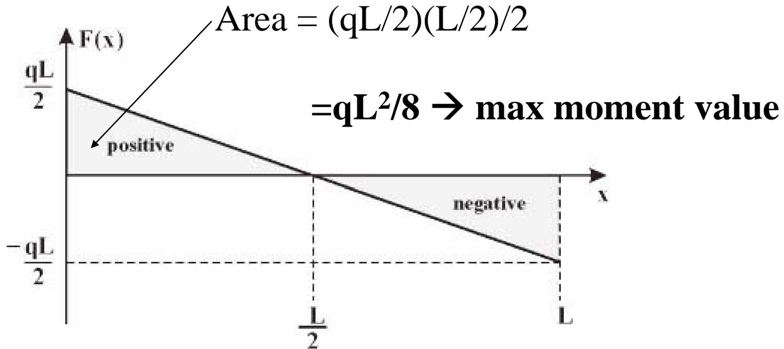
**Shear diagram equals the slope of moment diagram**
