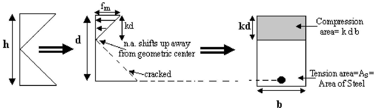
Concrete must crack in order for the reinforcing steel to carry load
