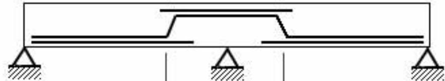
(d) Post-tensioned beam. Cable is draped to reflect moments present.
