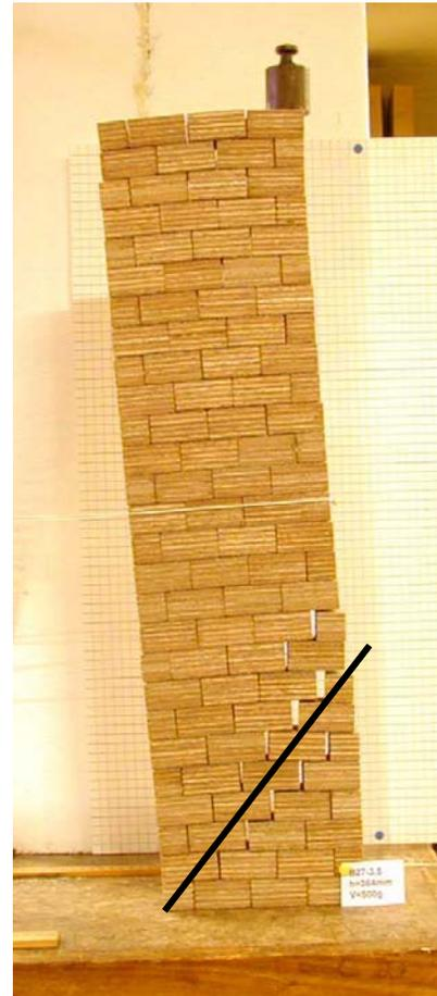
**Fracture reduces thrust capacity by 20% to 30%**
