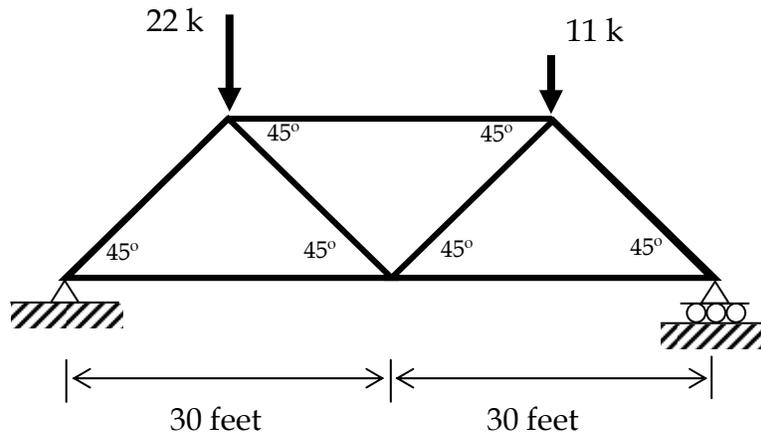
2) Using results from above, which element has the highest compression force? Design this element so that the safety factor against buckling is at least 3.0 due to the applied loads. You may assume that the element is pinned at each end.
