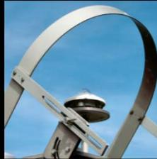
shadow band pyranometer
