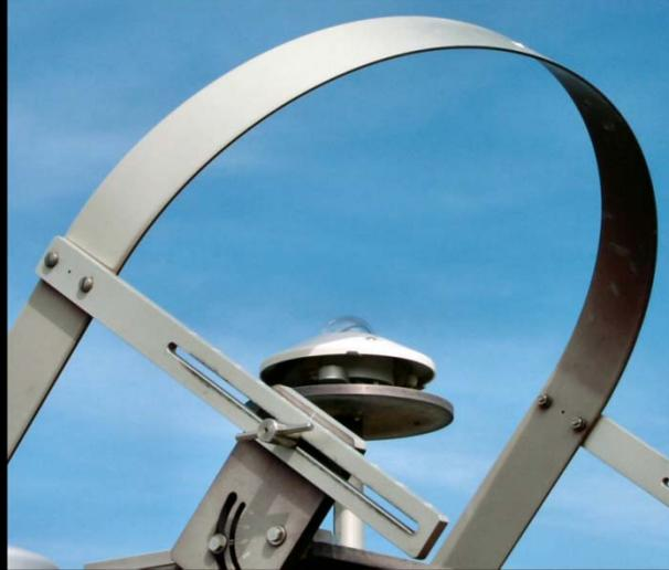
Source: Quaschnig, Volker. "Pyranometer with Shadowband."
