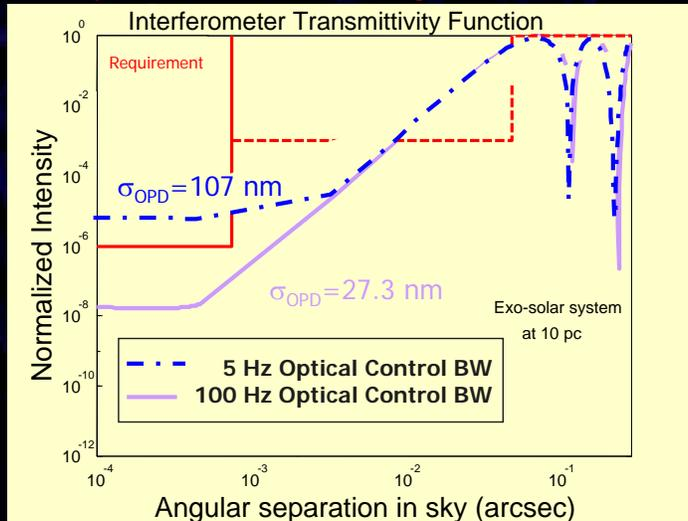
Trade study shows that optical control bandwidth is insufficient at 5 Hz but can meet the requirements at 100 Hz
