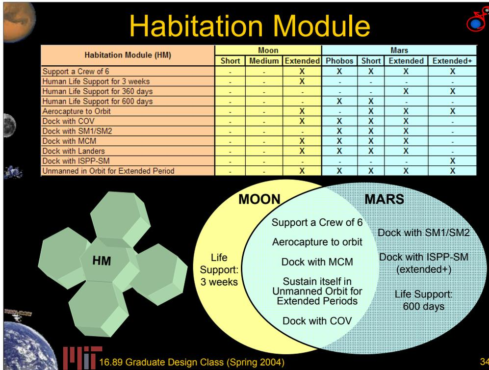
**ISPP-SM** = In-situ Propellant Production – Service Module
