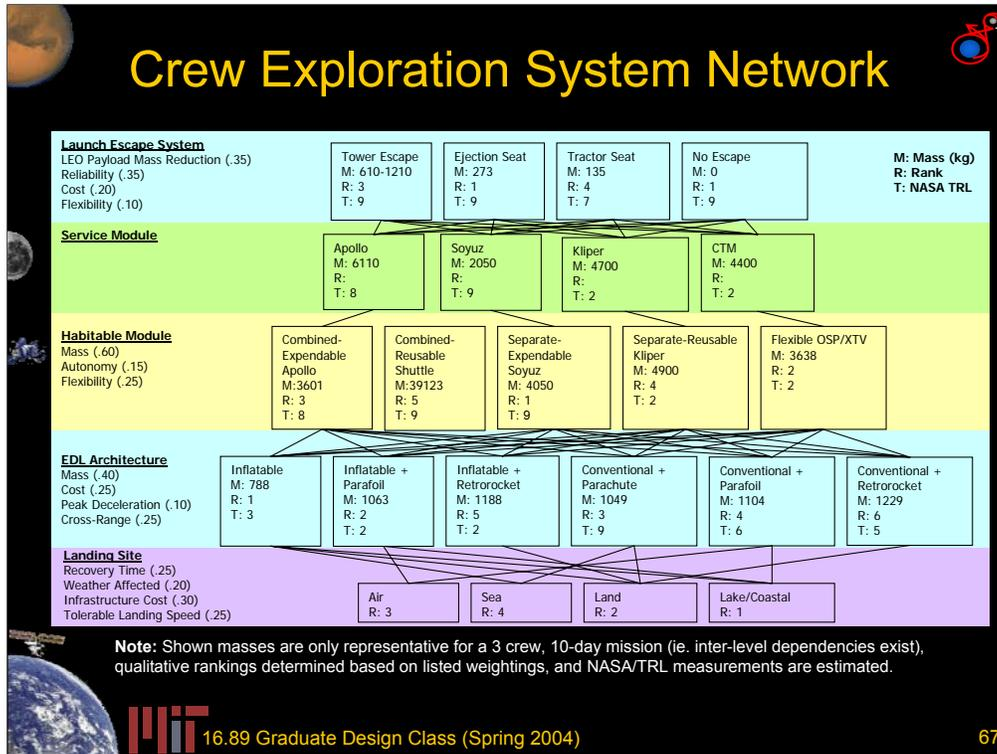
Emphasize that inter-level dependencies exist (eg. mass of reentry system depends on habital module). Links between levels represent preferable or feasible options. For example, the lake/coastal landing site option requires a reentry system with a large cross-range capability for precisely landing into a small body of water (inflatable or parafoil). More information provided in the EDL (entry, descent, and landing) and Landing site slides.
