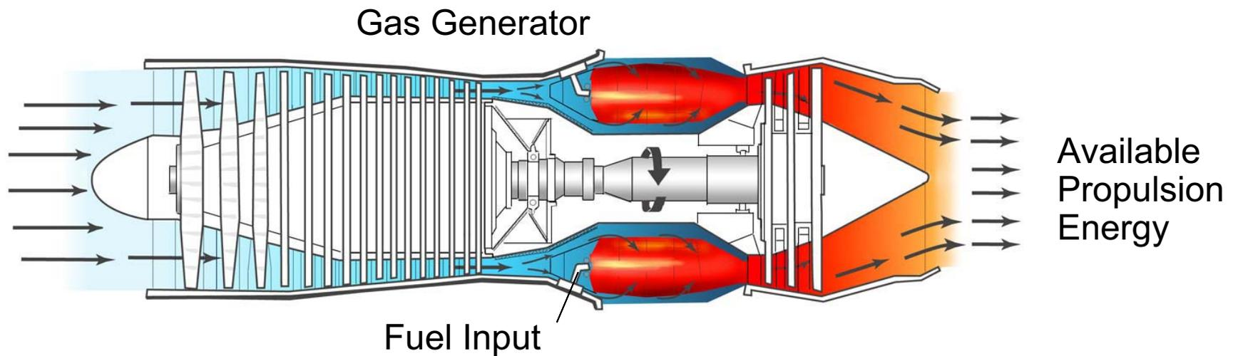
$$\eta_{\text{overall}} = \eta_{\text{thermal}} \times \eta_{\text{propulsive}}$$
