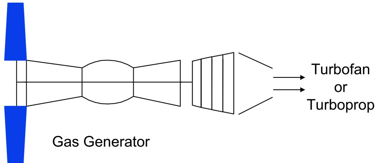
$\eta_{\text{propulsive}} \rightarrow 100\%$  as  $V_{\text{exhaust}} \rightarrow V_0$
