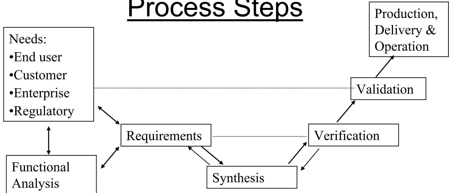
Systems engineering process is applied recursively at multiple levels: system, subsystem, component.
