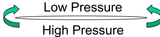
Kinetic energy in freestream redistributed to cross flow. It represents an unrecoverable loss called drag due to lift, or induced drag.
