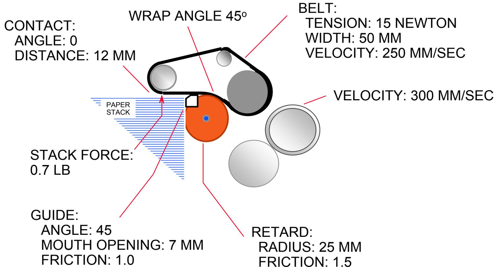
**Optimized values of critical parameters guide the detailed design**
