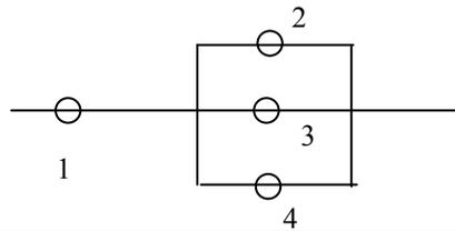
This system will fail if subsystem 1 fails *or* if subsystems 2,3, *and* 4 fail.
