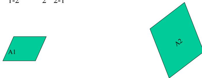
The view factor is a function of the size, geometry, relative position, and orientation of two surfaces.
