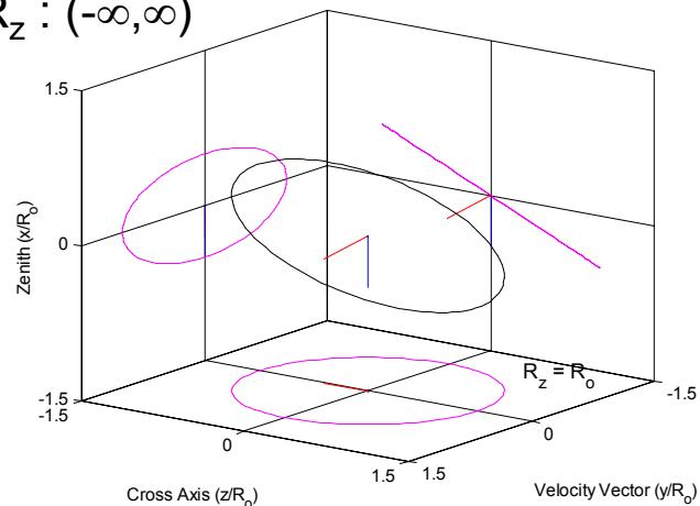
Intersection between a plane and a circular paraboloid results in an ellipse
