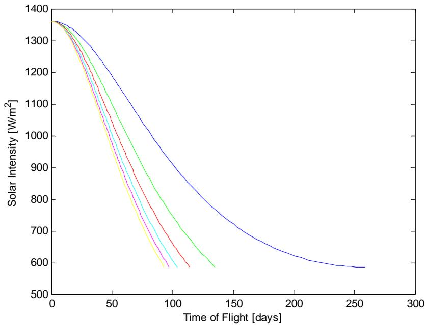
Figure 7. Solar power intensity for transfer orbits ranging from Hohmann transfer to a high energy transfer with 2.5 AU semi-major axis.
