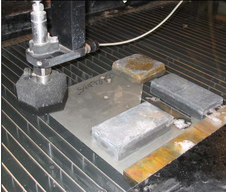
Figure 45 Water level raised - ready to begin machining
