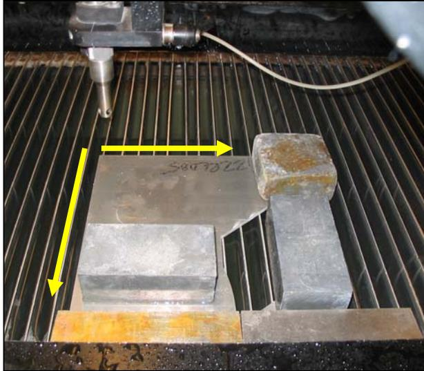
**Figure 42 Nozzle positioned at desired (0,0) location (home)**
