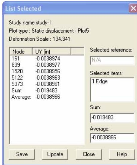
Figure 21 "List Selected" dialog box displaying node displacements
