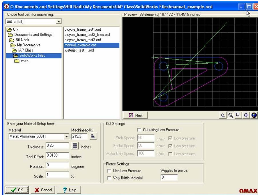
**Figure 36 Omax Make "Change Part Setup" dialog box**
