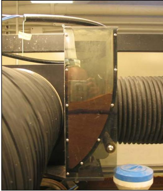
**Figure 39 Abrasive container for water jet cutter**
