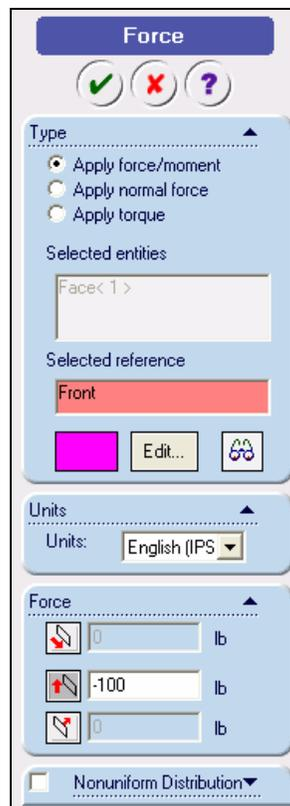
**Figure 10 Force dialog box for load on 2-D part**
