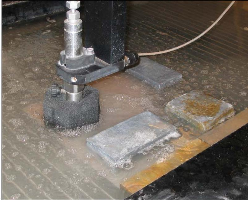
**Figure 47 Water jet cutter in operation**
