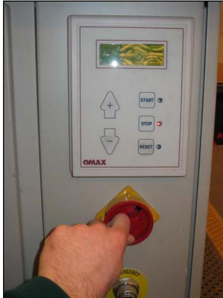
**Figure 35 Turning on/off power to water jet cutter**
