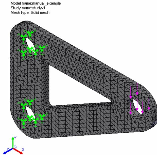
**Figure 14 Mesh result with restraints and loads displayed**
