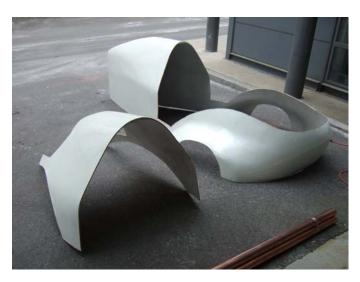
Marking an accurate curve on the existing shell was the hardest part of the manufacturing process; we carefully aligned the rails and used them to draw a curve on one side, extending it by eye to the nose of the vehicle. A grid was then created on the shell using masking tape and string to accurately reproduce this curve on the opposite side.
