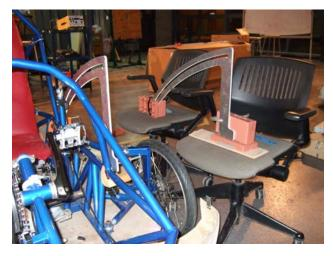
The rails were designed to be cut on a waterjet, as the complicated curving shape was too difficult to cut by hand and too large for the mill.
