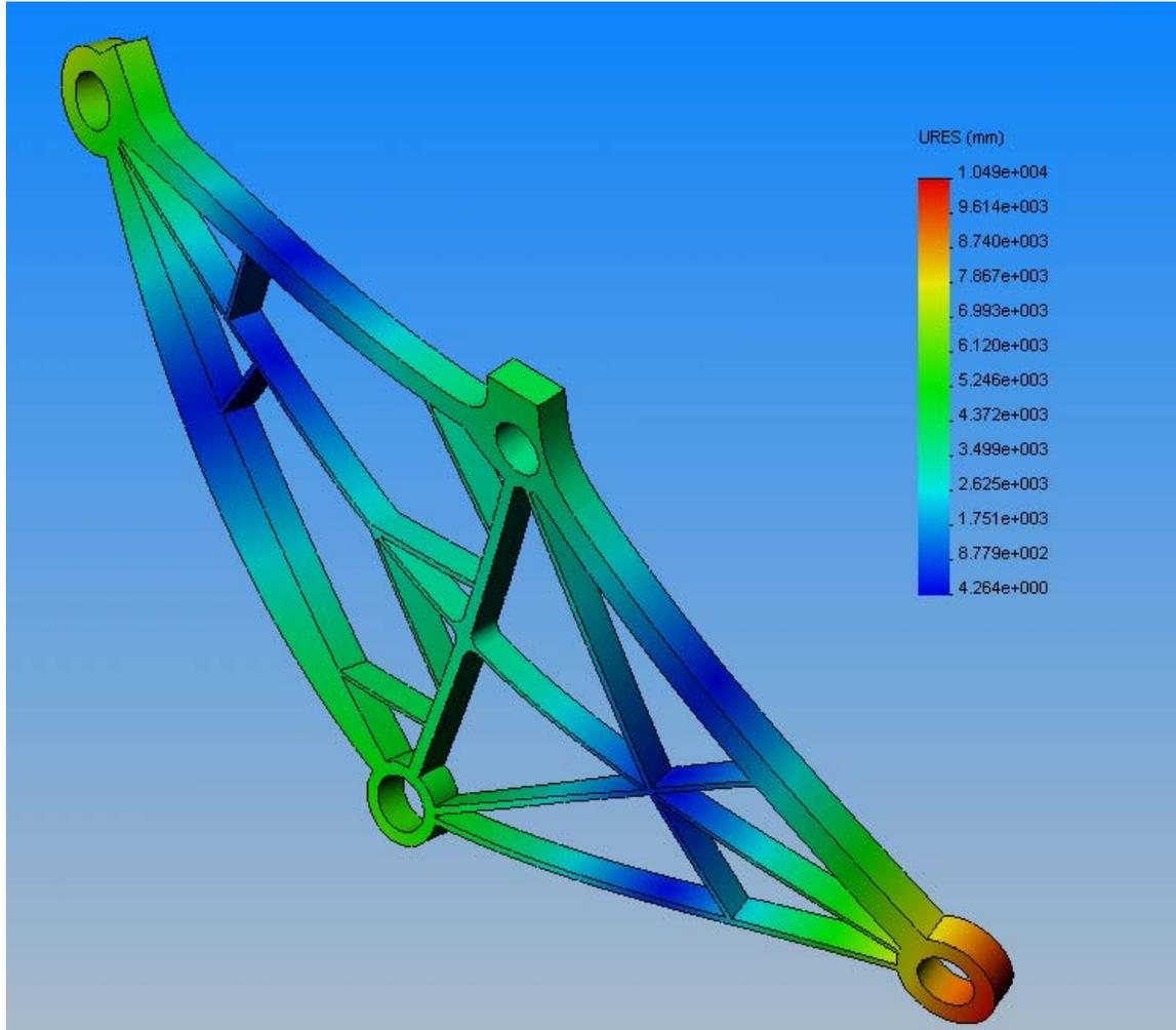
Figure 1: Mode Shape 1 @ 460 Hz of Version 1 for Team 5
