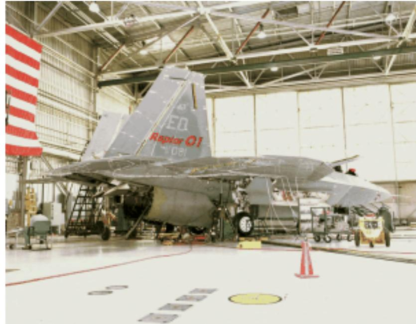
F-22 Raptor #01 during ground vibration tests at Edwards Air Force Base, Calif., in April 1999
