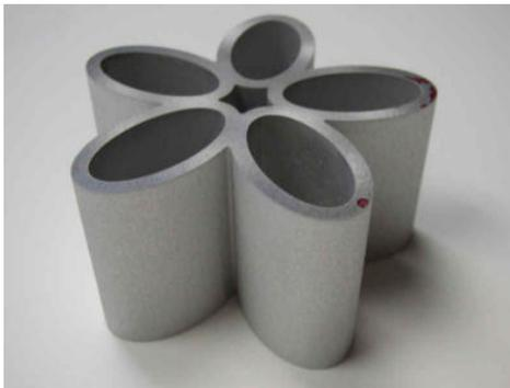
*A part machined from 3" (7.6 cm) aluminum; Intelli-MAX software lets you get sharp corners without wash-out*
