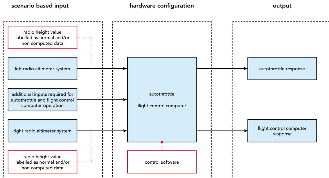
Illustration 17: diagram of the automatic flight system investigation
