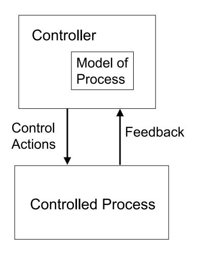
Accidents occur when model of process is inconsistent with real state of process and controller provides inadequate control actions
