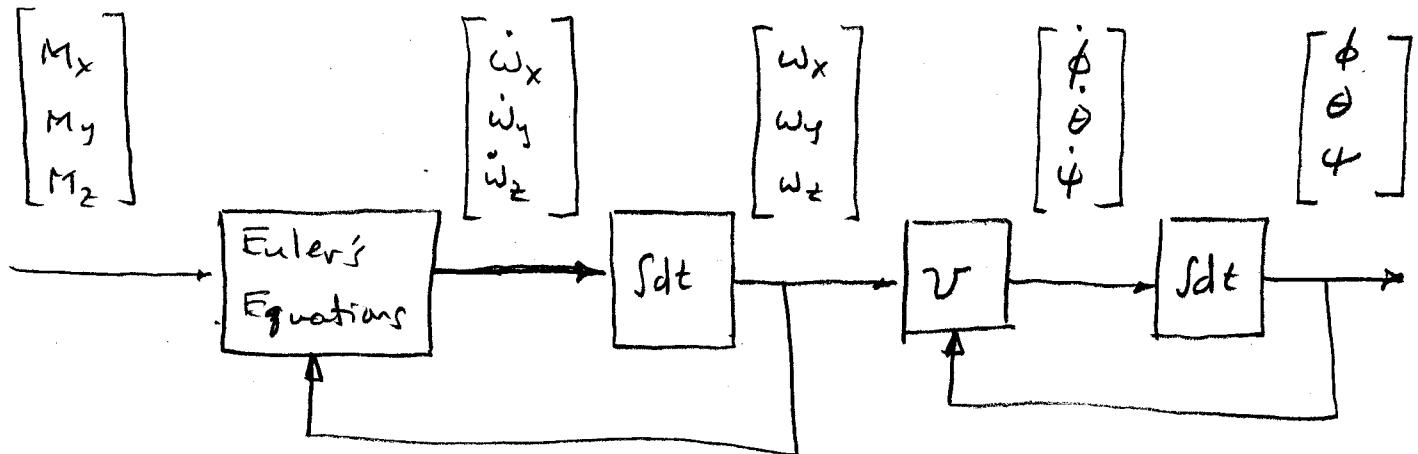
Both Euler's equations and the  $V$  matrix are nonlinear. Typically a S/C would have an inertial system and external sensors (e.g. star trackers) to determine the angular velocities and the attitude. The system has six state variables  $\phi, \theta, \psi, w_x, w_y, w_z$ , all of which are measured by the sensors and can be fed back to a controller.
