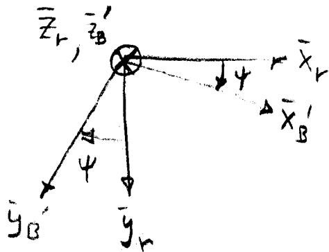
$$T_3(\psi) = \begin{bmatrix} c\psi & s\psi & 0 \\ -s\psi & c\psi & 0 \\ 0 & 0 & 1 \end{bmatrix}$$
