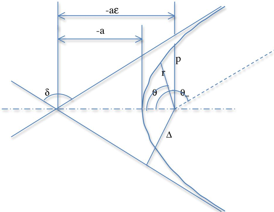
The “parameter”  $p$  still has the geometrical significance indicated in the figure, and is therefore a positive number. It is still related to  $a$  and  $\epsilon$  through  $p = a(1 - \epsilon^2)$ , but now  $a$  is a negative number, so it is  $(-a)$  that has a geometrical significance, as indicated in the figure. Note also that  $\epsilon$  is still defined as the ratio of the distance from periapsis to center to the distance from focus to center.
