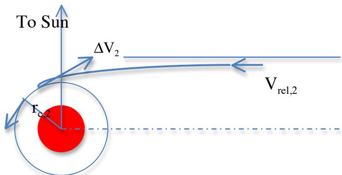
Just before the insertion rocket firing, the energy per unit mass relative to planet 2 is equal to  $\frac{1}{2} (v_{rel,2})^2$ , and it is also equal to the sum of the kinetic energy at that point of closest approach, plus the potential energy:  $\frac{1}{2} (v_{closest\ app.})^2 - \frac{\mu_2}{r_{c2}}$ . Thus we must have
