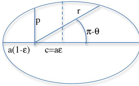
With reference to the figure, the polar equation of the trajectory is  $r = \frac{p}{1 + \epsilon \cos \theta}$ ,
