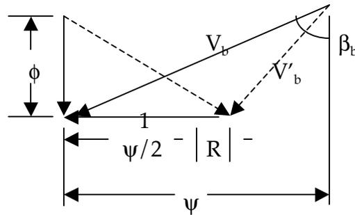
Drawing the velocity triangles for  $R=1/2$  (called 50% reaction) and for  $R=0$  (called Impulse),
