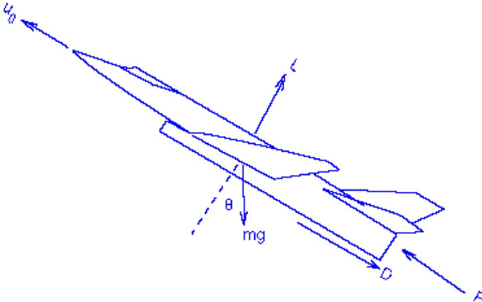
Suppose the aircraft is climbing at angle  $\theta$  from the horizontal. The equation of motion along the path is
