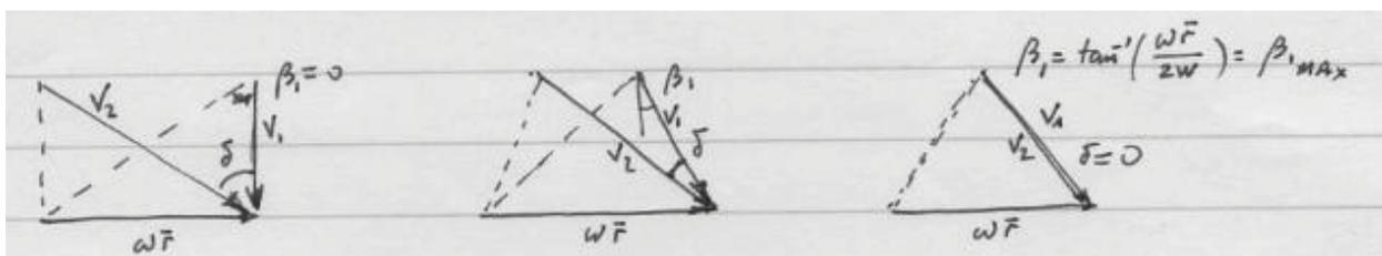
It is clear that as  $\beta_1$  increases (left to right),  $\delta$  decreases. So, the smallest  $\beta_1$  angles give the highest blade loading (most flow turning).
