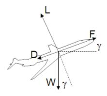
Force balance along and transverse to the trajectory:
