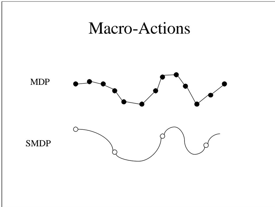
This is a graphical representation of how primitive actions compare to macro-actions in an MDP. While primitive actions cause the MDP to step through each state, using macro-actions across longer lengths of time, we are able to reduce the complexity of the problem.
