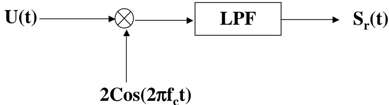
$$U(t)2\text{Cos}(2\pi f_c t) = 2S(t)\text{Cos}^2(2\pi f_c t) = S(t) + S(t)\text{Cos}(4\pi f_c t)$$
