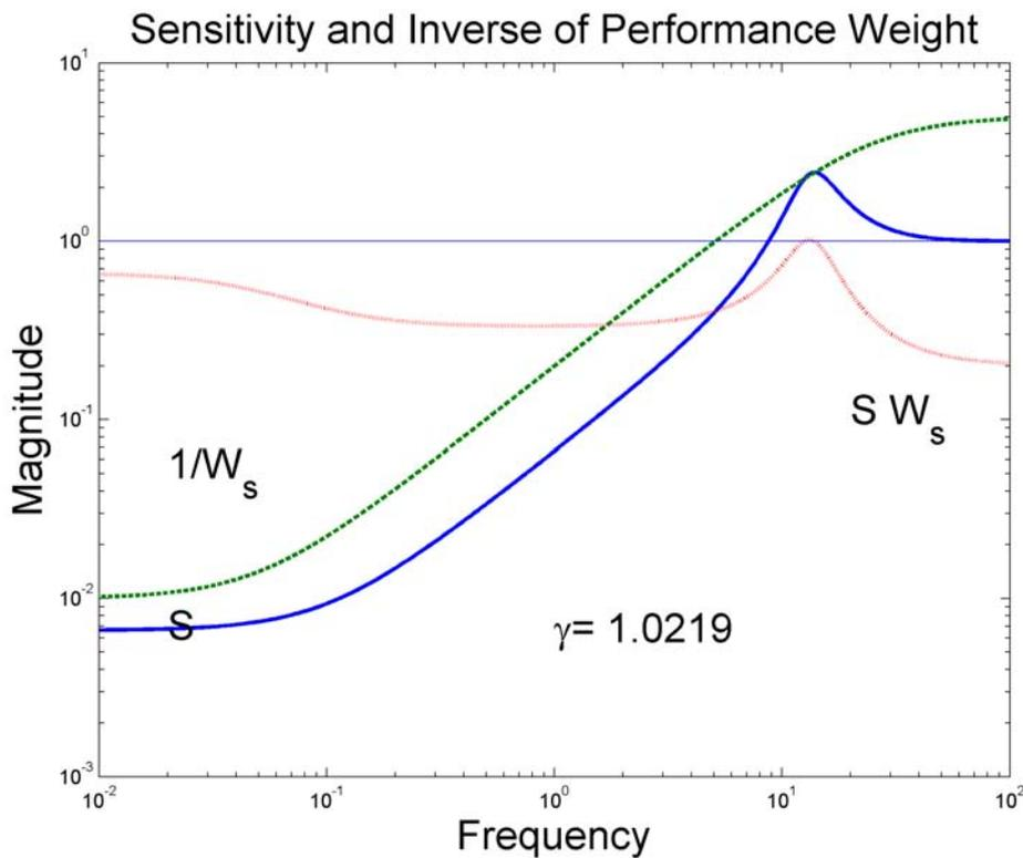
Fig. 2: Want  $|SW_p| < 1$ , so we just fail the test
