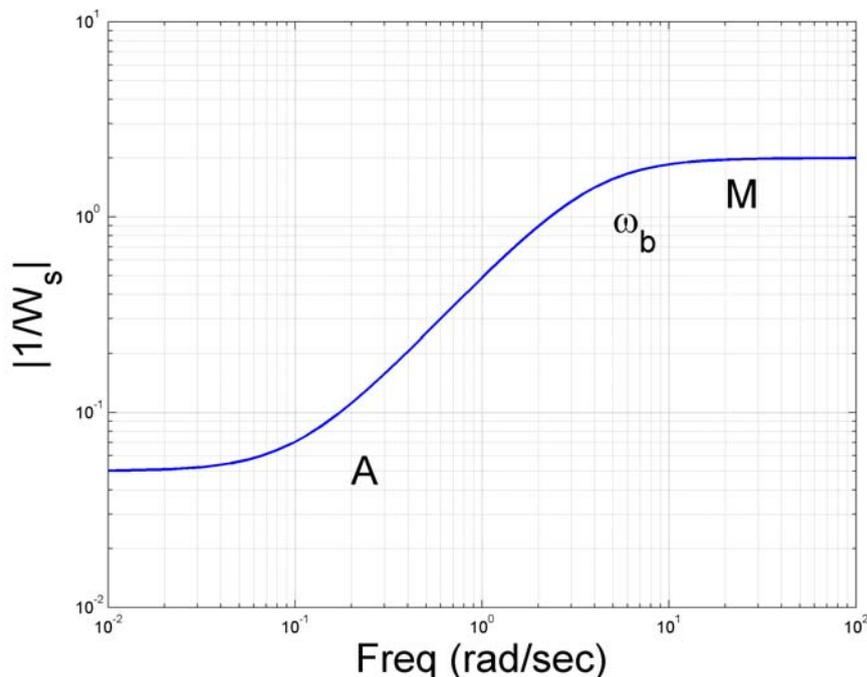
Fig. 1: Example of a standard performance weighting filter. Typically have  $A \ll 1$ ,  $M > 1$ , and  $|1/W_s| \approx 1$  at  $\omega_B$
