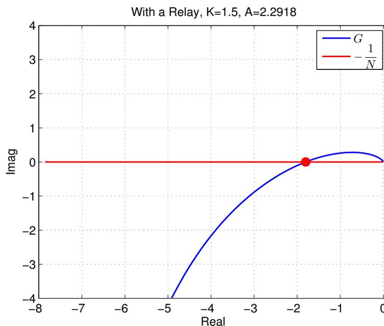
Fig. 1: DF graphical test – note that the DF is on the negative real line, parameterized by  $A$ , whereas the transfer function of  $G$  is parameterized by  $\omega$
