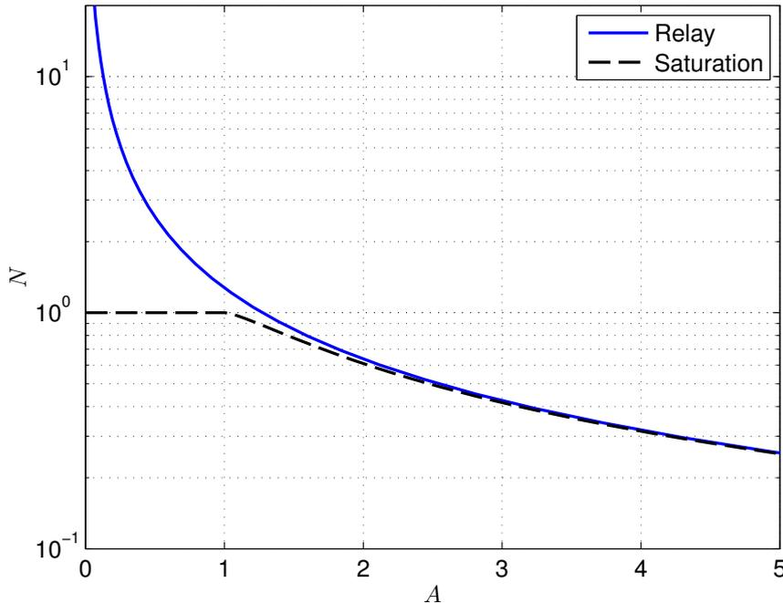
Fig. 4: Comparison of  $N$  for relay and saturation
