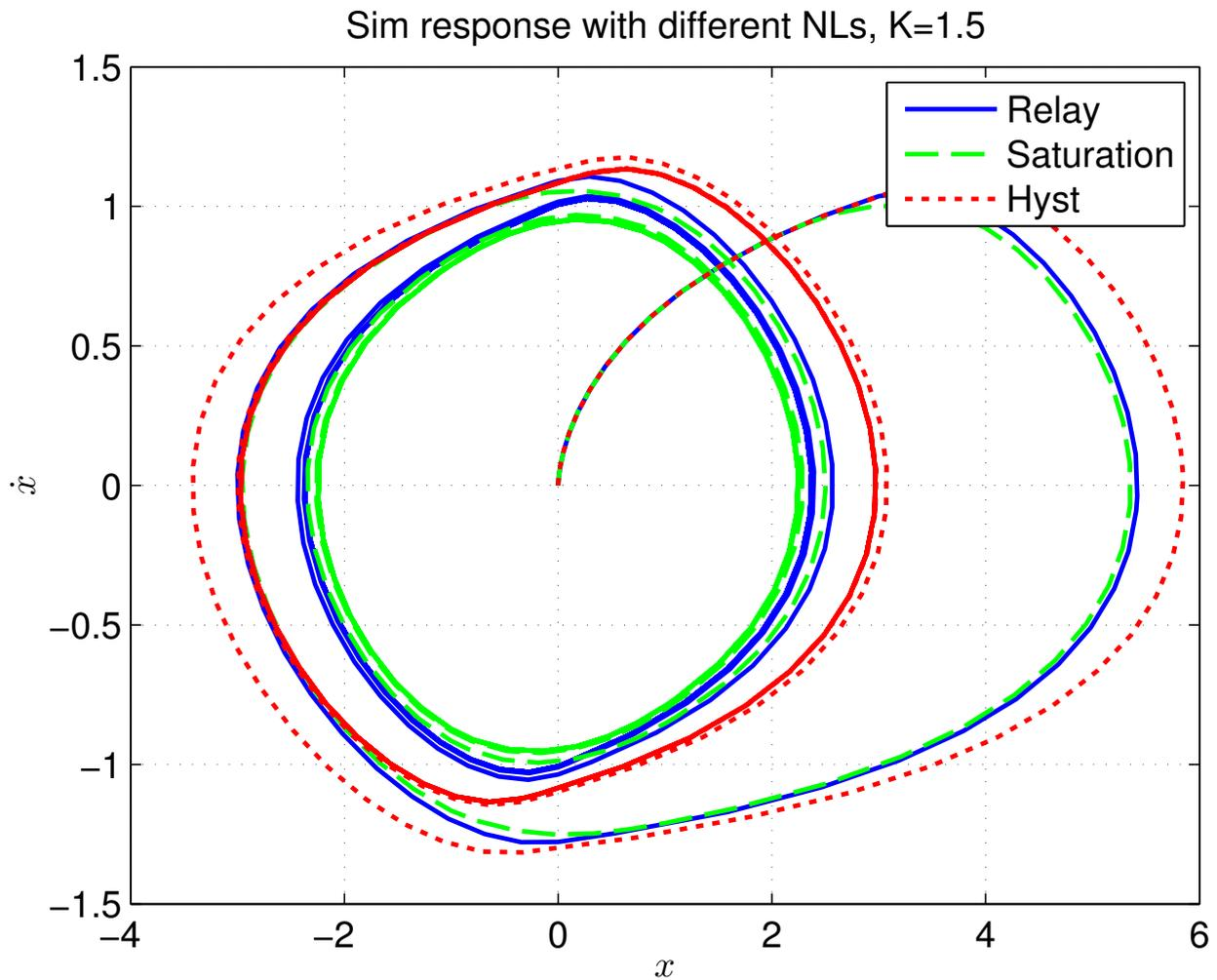
Fig. 6: Simulation comparison of all 3 types of nonlinearities with  $K = 1.5$ . Simulation results agree well with the predictions.
