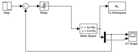
Fig. 2: Typical simulation setup
