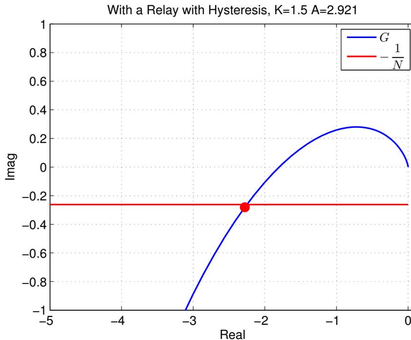
Fig. 5: Test for limit cycle for a relay with hysteresis,  $K = 1.5$ ,  $\Delta = T/3$
