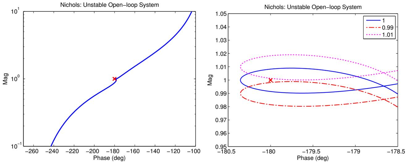
Fig. 4: Nichols Plot ( $|L(j\omega)|$  vs.  $\arg L(j\omega)$ ) for the cart example which clearly shows sensitivity to overall gain and/or phase lag.
