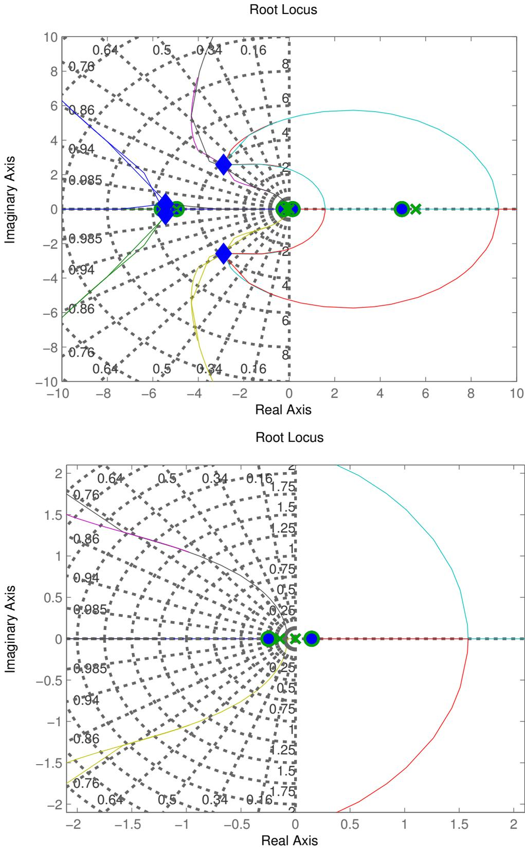
Fig. 3: Root Locus with frozen compensator dynamics. Shows sensitivity to overall gain – symbols are a gain of [0.995:0.0001:1.005].
