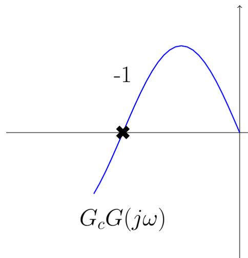
Fig. 8: Polar plot of a neutrally stable case
