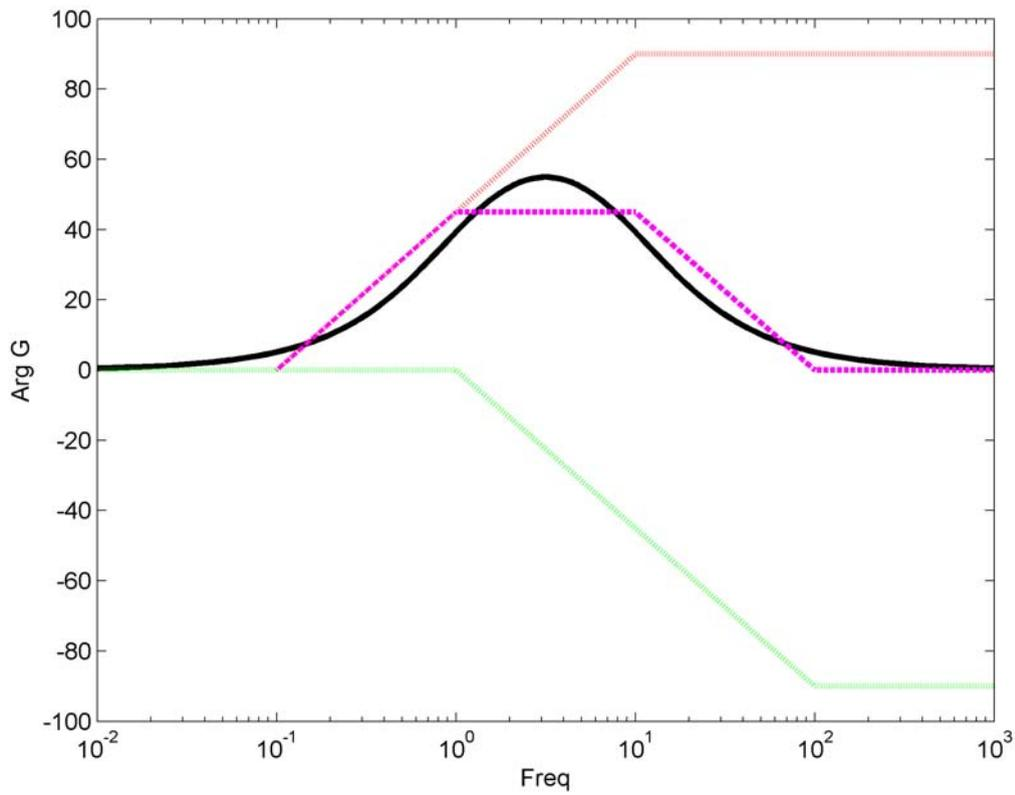
Fig. 4: Phase plot  $G(s) = 10(s + 1)/(s + 10)$  which is a “lead”.
