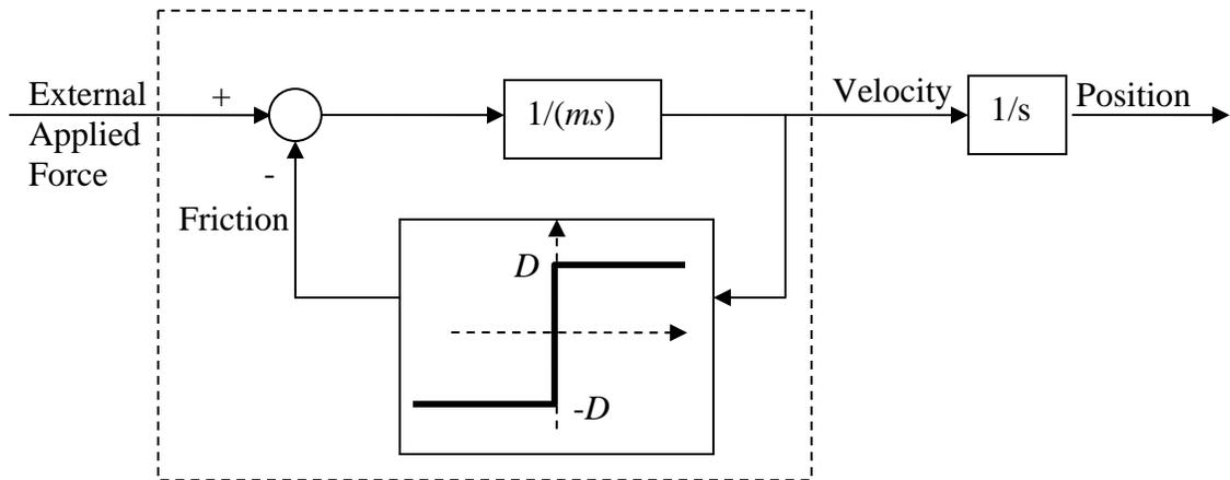
In this diagram, the dry friction maximum amplitude is  $D$ . For all numerical calculations, assume  $D=1$  and  $m=1$ .
