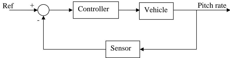
The sensor is represented by a gain  $H(s)=0.5$ , and the vehicle is represented by the transfer function
