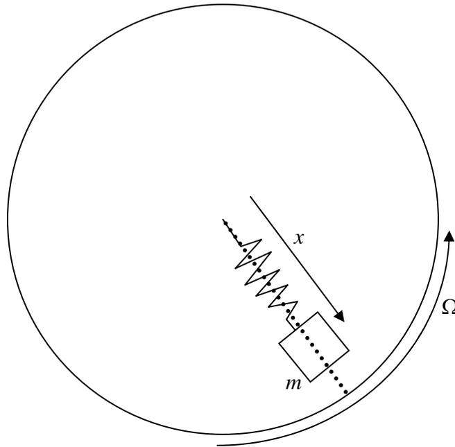
A mass  $m$  is mounted on a disk in such a way that it can slide (with no friction) only along a groove (dashed line) rigidly attached to the disk. This mass is connected to the center of the disc by a softening spring. The characteristic of the spring is given in the figure below; it is symmetric with respect to the origin:
