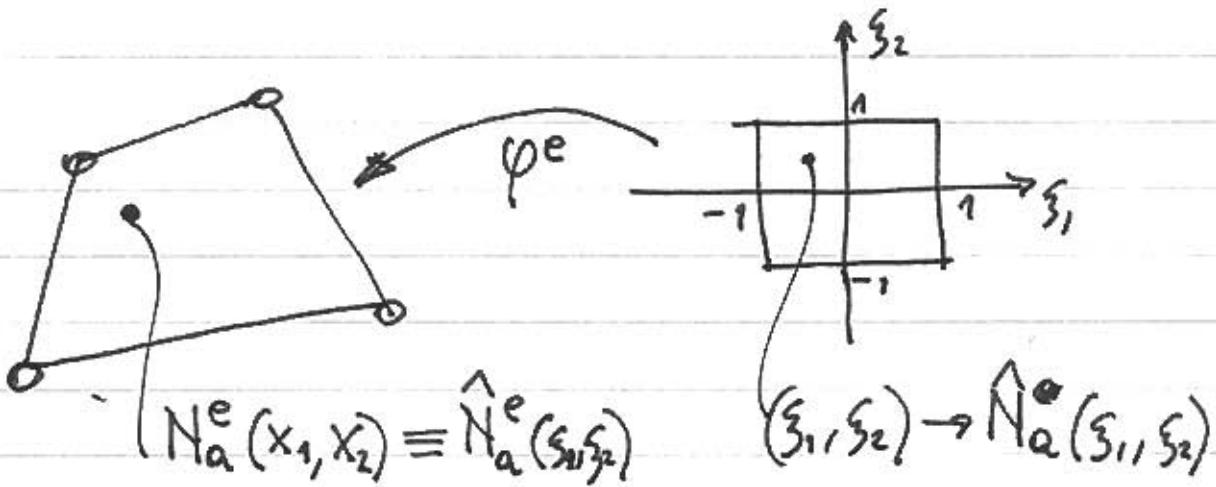
$$N_a^e(x) = \hat{N}_a(\underbrace{\varphi^{-1}(x)}_{\xi}) = \hat{N}_a \circ \varphi^{-1}$$
