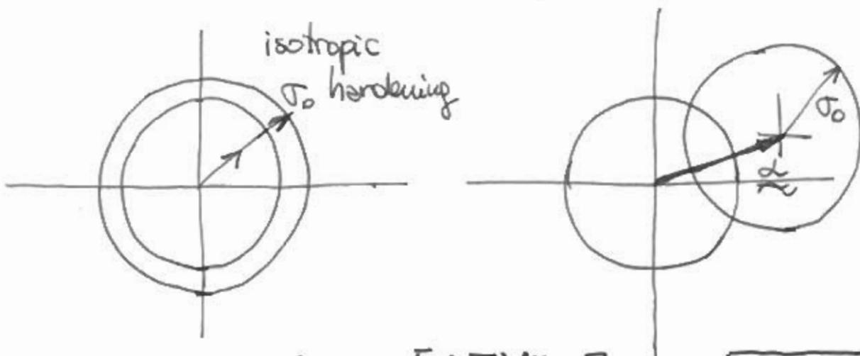
Isotropic:  $\phi = \frac{\sigma_y}{\eta} \left[ \left( \frac{\bar{\sigma}}{\sigma_0} \right)^m - 1 \right], \bar{\sigma} = \sqrt{\frac{3}{2} \bar{s}_{ij} \bar{s}_{ij}}$
